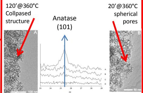
Center: X-ray Diffractograms of ST films calcined at different temperatures (heating ramp 1°C/min): A: 2h@360°C, B: 20min@360°C, C: 10min@360°C, D: 2h@350°C.
